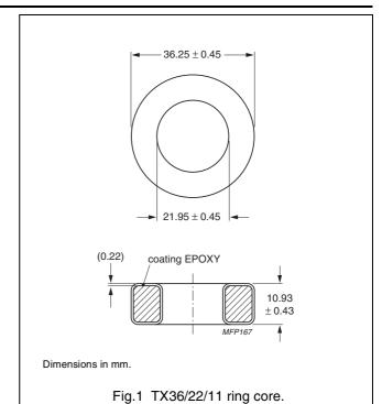
**Ring core data - Note** 1. Mechanical dimensions : OD  $\leq$  36.63, ID  $\geq$  21.54, H  $\leq$  11.28
